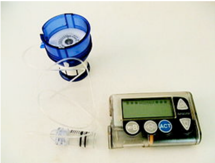
Insulin pump, showing an infusion set loaded into spring-loaded insertion device. A reservoir is attached to the infusion set (shown here removed from the pump). (Public Domain; User:David-i98 ).
