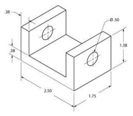
Directions: on a separate piece of paper, make a dimensional orthographic sketch of the object.
