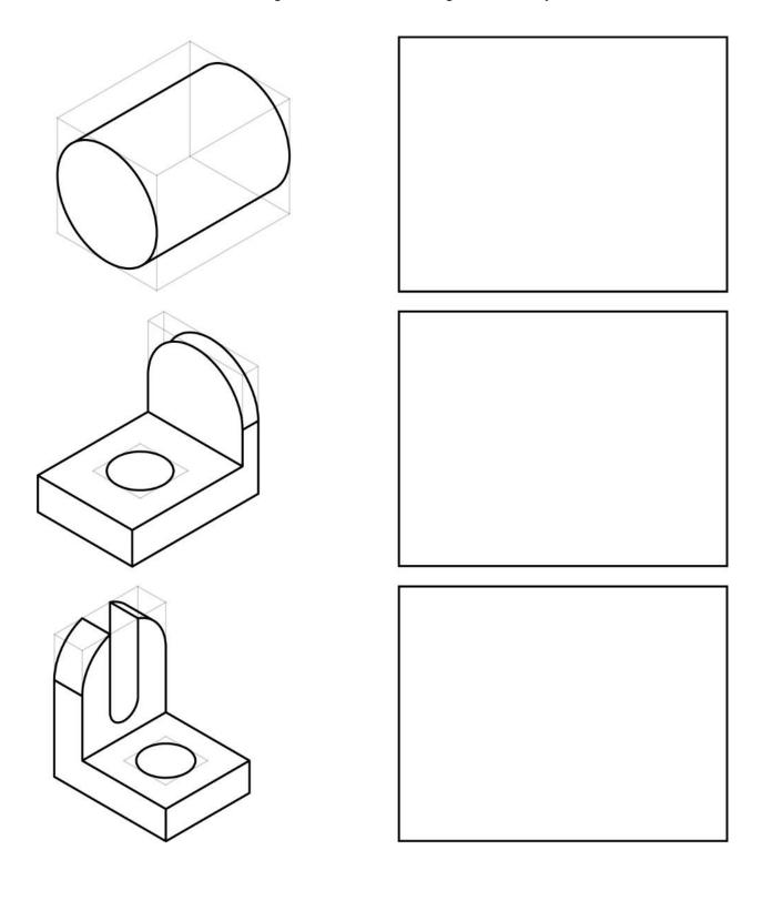
Directions: Sketch isometric drawings into the boxes on the right for each object.
